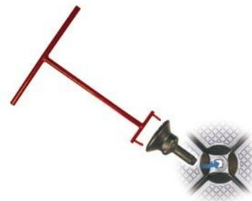
A connecting pin is inserted into the holes of the over-lapping lugs and locked into place. A 45° turn of the pin with the Jetfloat Assembly Key will lock or unlock the Jetfloats. (The dock cannot be disassembled without the key.)
